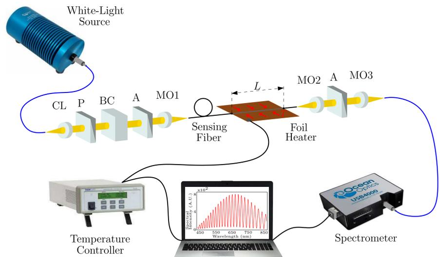
**Figure 7:** Experimental setup with HB sensing fiber to measure temperature with utilizing of the Vernier effect; collimating lens (CL), polarizer (P), birefringent crystal (BC), analyzer (A), microscope objectives (MO1 - MO3).
