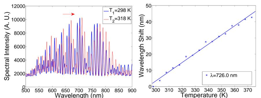
**Figure 8:** Recorded spectra with envelopes for temperatures  $T_1$  and  $T_2$ .
