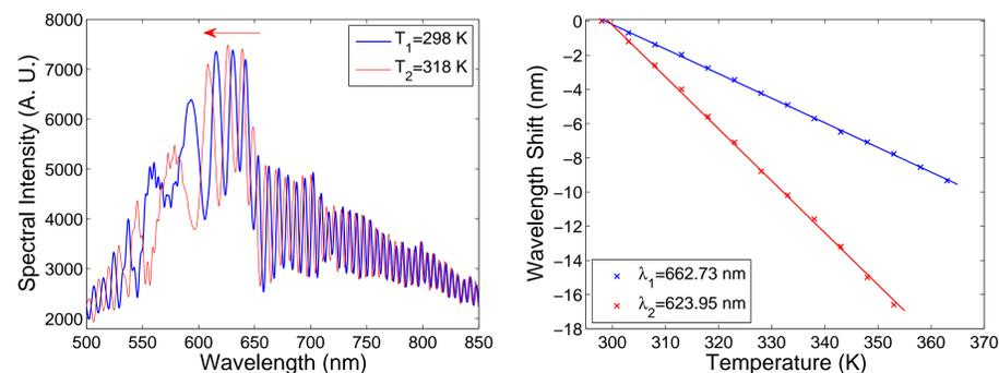
**Figure 5:** Recorded spectra with equalization wavelengths for temperatures  $T_1$  and  $T_2$ .
