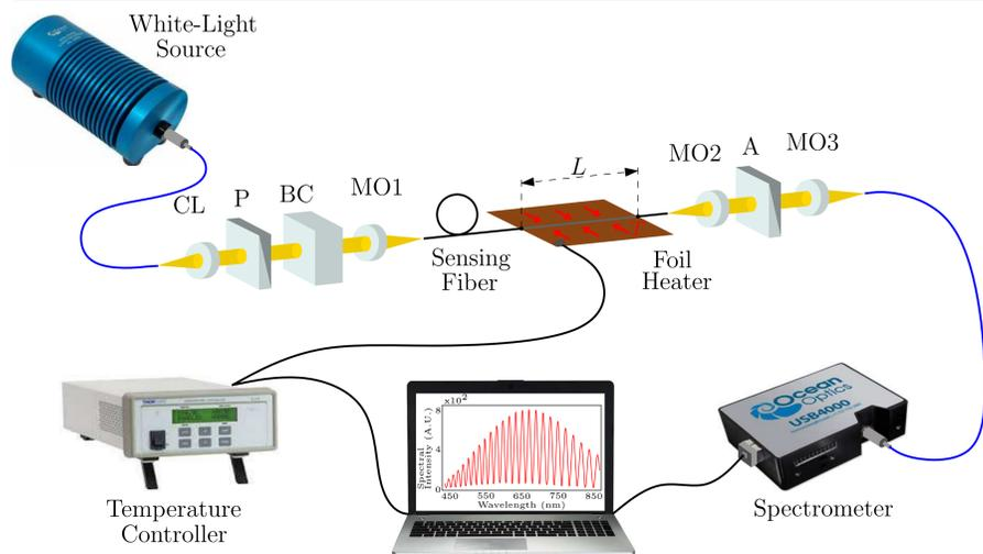
**Figure 4:** Experimental setup with HB sensing fiber to measure temperature with higher sensitivity; collimating lens (CL), polarizer (P), birefringent crystal (BC), analyzer (A), microscope objectives (MO1 - MO3).
