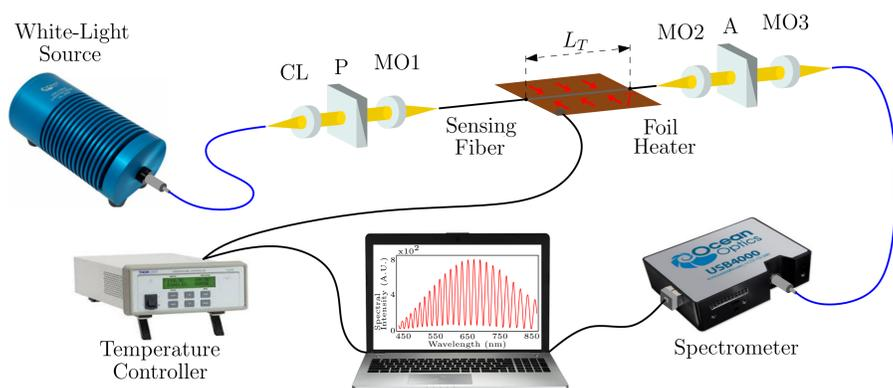
**Figure 1:** Experimental setup with HB sensing fiber to measure temperature; collimating lens (CL), polarizer (P), analyzer (A), microscope objectives (MO1 - MO3).
