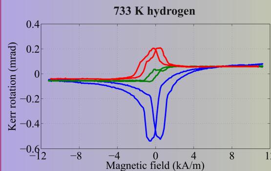
blue, red, and green loops correspond to the case, when light is focused into the different places on the ribbon surface, magnetic field applied along H<sub>4</sub> direction
