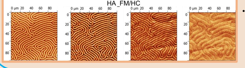
the distance  $d_z$  between the probe and sample surface is 25 nm, 300 nm, 1000 nm, and 2000 nm.
