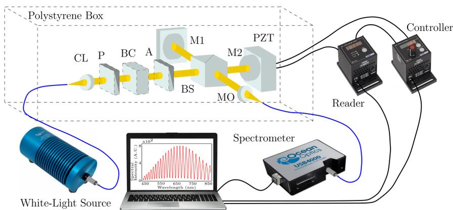
**Figure 1:** Experimental setup with a Michelson interferometer to measure mirror displacement; collimating lens (CL), polarizer (P), birefringent crystal (BC), analyzer (A), beam splitter (BS), mirrors (M1, M2), piezo transducer (PZT) and microscope objective (MO).
